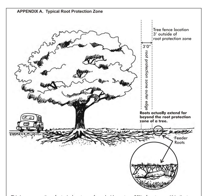
This is a cross section of a typical root zone for a deciduous tree. 85% of roots are within the top 18" of the soil. Roots spread amazingly far from the trunk. They typically spread up to 2 times the height of the tree and sometimes farther! However, the essential mass of roots is usually found within the **ROOT PROTECTION ZONE**.
